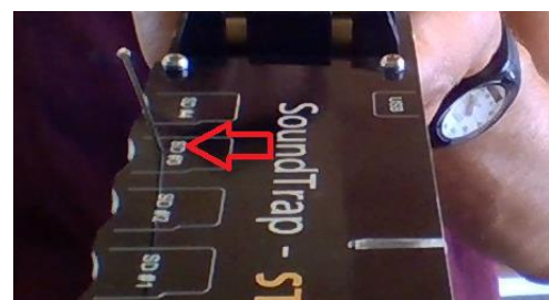
Figure 4 - Location of reset switch
