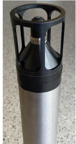
**Figure 2 – Avoid fouling of the locking screw by covering with insulation tape**
